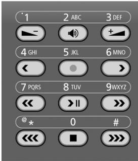
On the 19" model the numerical keys and the recorder keys are combined. This is possible because depending on the selected procedure the function of the keys is always obvious.
