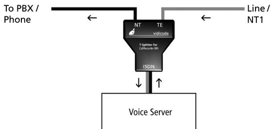
Per line you have received a T-splitter a long 8 wire ISDN cable and a short 8 wire ISDN cable.
